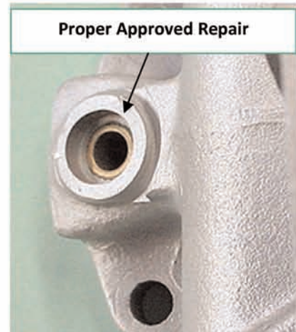
Figure 3: Proper Bushed Repair
