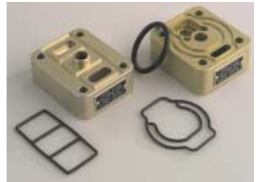
Pumps incorporating new valve housings manufactured by Crane/Romec are no longer subject to Lycoming SB 529. These relief valve housings rely on the improved sealing characteristics to eliminate fuel leakage and the need for repetitive torquing.
