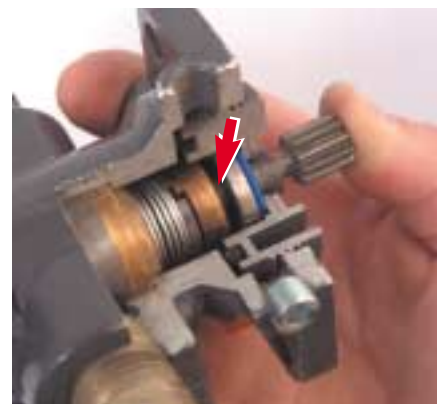
Do not depress the drive-coupling when handling or installing Lear Romec pumps. Depressing the coupling could allow contaminants to get between the disc and plate seal damaging the seal faces, and ultimately resulting in fuel leakage from the fitting at the base of the pump.
