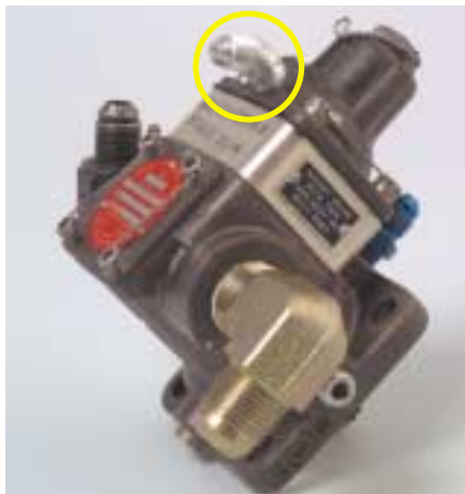
Textron Lycoming and Crane have issued numerous bulletins emphasizing the importance using orificed reference fittings. The type of fitting and orientation are determined by engine and airframe application. Orificed fittings are readily identified by an "R" stamped on the fitting. Lycoming Service Bulletins 487, 494, and 497 specify which fittings to use.
