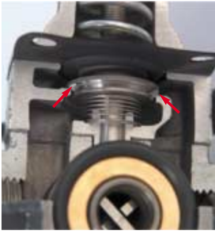
Contaminants trapped between the valve face and seating area can dramatically reduce pump output. Loss of pressure is more pronounced at idle speeds.
