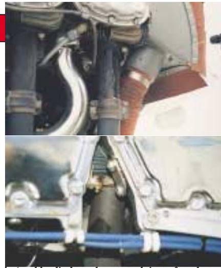
*A cold cylinder exhaust stack just after shut-down indicates the malfunctioning plug or injector. A small amount of water squirted on the stack will steam and possibly boil.*
