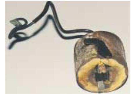
*Cracked and burned coils, such as that pictured here, will often show up only at altitude as altitude misses. Without an external damage indication, these can usually be found best by disassembly or bench check of the mags.*
