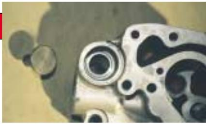
Any debris caught between the plunger and seat of the oil pressure relief valve (TCM newer style shown) will cause low oil pressure with hot oil but not with cold. When the oil is hot, pressures at idle can even drop below redline. This is true for any abnormal/excessive internal oil leakage. If cleaning the plunger and seat doesn't help, or if the debris is metal, further investigation is definitely warranted.
