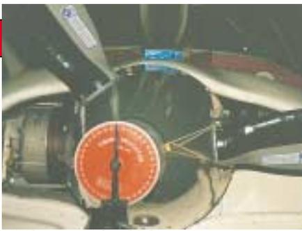
*“Flower pot” for checking magneto to engine timing. Inaccurate timing can give excessive mag drops or high cylinder head temperatures. This is also the preferred timing check method for Continental engines per TCM.*
