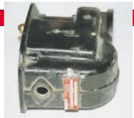
*External damage to a magneto caused by chaffing screw and aggravated by internal arcing and burning of the coil.*
