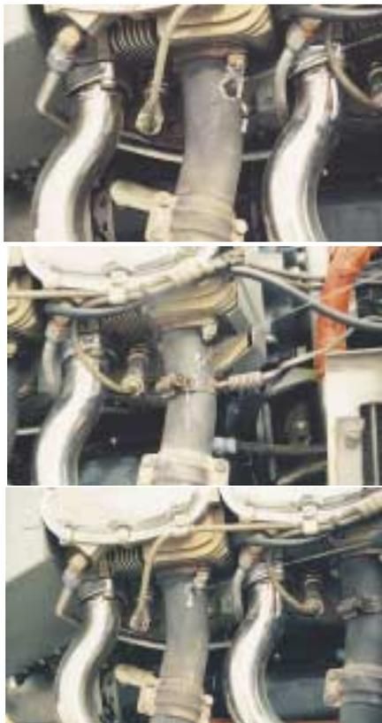
*A small amount of water squirted on firing cylinder's exhaust stack will ball, sizzle, and immediately fall off stack.*
