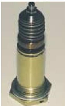
This near new "Vernatherm" was the culprit in oil temperature problems. Upon removal and inspection there is usually no external indication of a problem unless the valve face is excessively worn. A new vernatherm solved the problem immediately.
