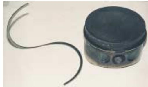
Annealed rings, caused by piston overtemp, will give high oil consumption and, in advanced stages, low compression. Notice the oil burned and blackened piston. If the top compression ring can be twisted to take a set at or more than 90 degrees without breaking, it is generally considered annealed. The usual culprits of piston overtemp are lean mixtures at high power settings (70 percent or higher) or partially clogged fuel nozzles.
