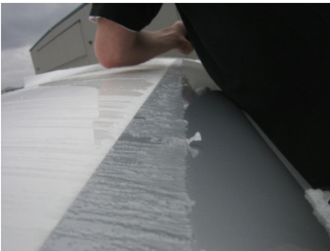
The ThermaWing De-ice System Minimizes Runback
