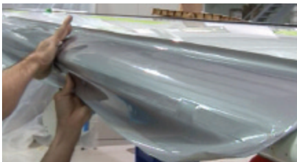
Installing the ultra-thin lightweight graphite foil
