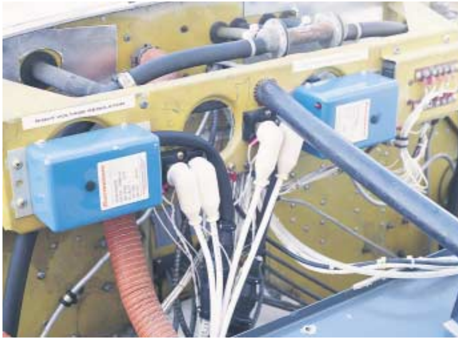
Paralleling remains the most challenging aspects of installing alternators or regulators in twin-engine applications.
