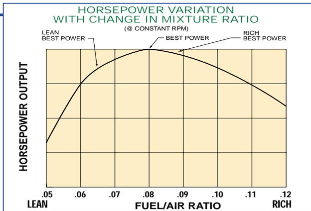
*This curve shows the relationship between power output and mixture ratios (based on weight, not volume). Combustion can occur with mixtures as rich as .125 (1 to 8); and as lean as .062 (1 to 16). Lean best power (economy) setting is 0.075, while rich best power is 0.087. Best performance is approximately 0.080. The exact shape of this curve varies from engine to engine.*
