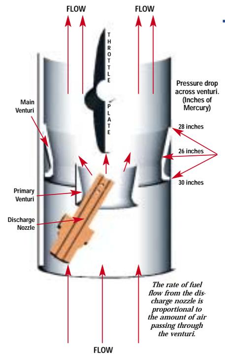
unsteady or turbulent airflows directly affecting the fuel metered through the discharge nozzle. The quality of the airstream directly influences the metering of fuel. A small piece of gasket material, a damaged or restricted air filter, a loose venturi, or any foreign object lodged in the carburetor throat can ruin the metering ability of the carburetor.
