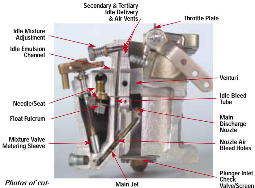
*Photos of cut-away views of MA-4SPA Carburetor. Model shown is typically installed in Textron Lycoming O-320 series engines.*
