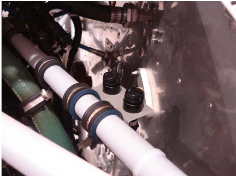
Figure 3 – Suggested Installation of AC-00107 Fuse Holder Bracket (Adel Clamps/hardware procured locally)
