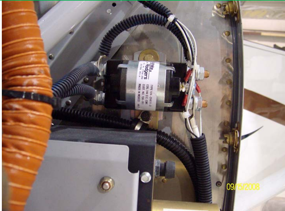
Figure 1- Mounting location of DC contactor relay.
